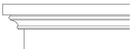
Top with Trim EST-CH Adds 1" to overall height. Adds 2" to overall width.
