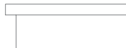
Top with ¾" Overhang EST-TR Adds 1" to overall height. Adds 1½" to overall width.
