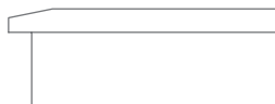
Top with Large Bevel EST-LB Adds 1" to overall height. Adds 1½" to overall width.
